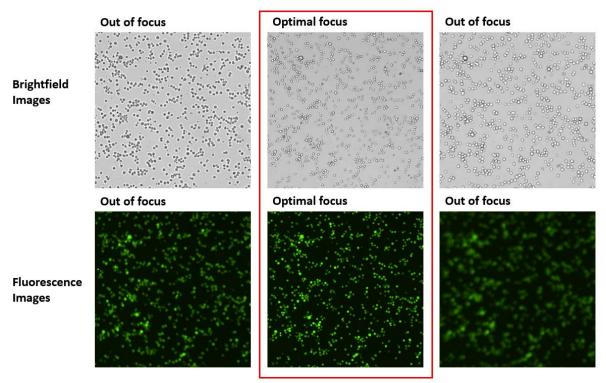
4.5.3. Once the sample is focused, click the **FL** button to preview Channel 1 fluorescence 4.5.3.1. Adjust exposure times as needed
