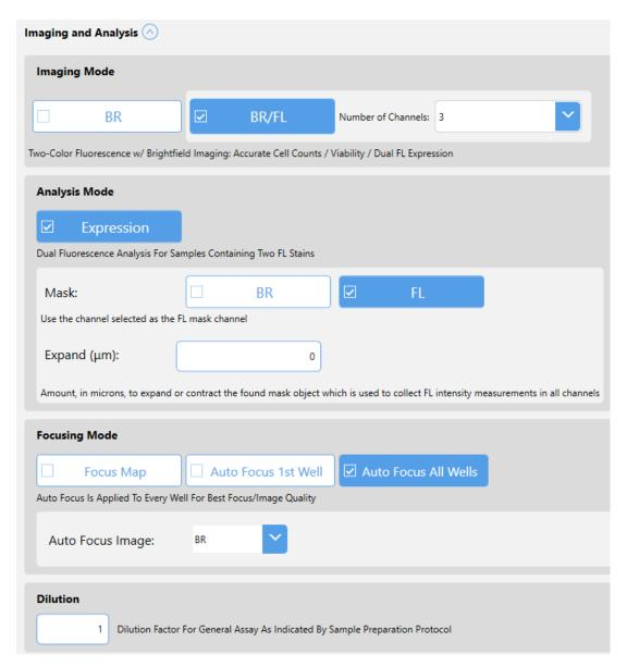
**NOTE**: Below are the default Imaging Parameters for each channel in the Cellaca® PLX, anti-human CD4 PE / CD8 APC Total Cell Kit
